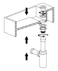
Hold basin against wall aligning outlet of trap with waste pipe. Extend telescopic trap up or down to find desired height & cut waste to suit trap.
