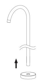
Push the spout onto the base plate and tighten the grub
