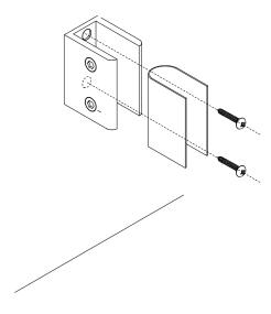
Install Glass. Can be used on glass up to 12mm thick. For panels less than 12mm thickness ABI recommends clear rubber packers to be used (supplied by others). Tighten up grub screws using an allen key. This will clamp the glass to hold it in place.
