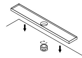
The remainder of the sand cement is installed to allow for correct falls down to the drain.
