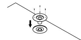
Adjust the top of the puddle flange to the finished height required for the shower grate installation.
