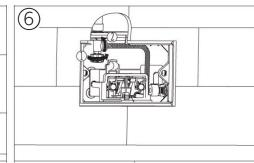
Remove hose by twisting anti-clockwise
