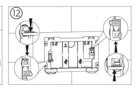
Hold button plate vertically and fit lock threads (4) into When plate (3) is in place, lock threads in by turning the cistern plate holes
